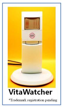
The "VitaWatcher" device was developed in collaboration with Dr. Takuya Sakamoto, professor at Kyoto University Graduate School of Engineering, and is intended to monitor the subtle body movement of a subject caused by the respiration and heartbeat in a contactless manner.
